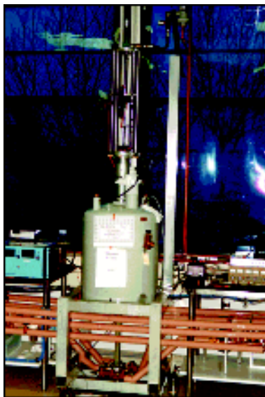
A magnetic refrigeration setup. (Courtesy Vitalij Pecharsky, Ames Lab/University of Iowa.)
